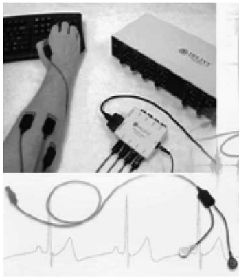
Fig. 8. EMG sensors are placed so as to inform about particular muscle group activity.
